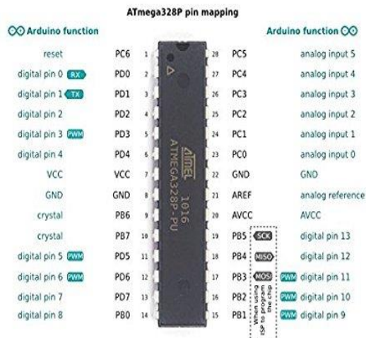
Figure 2. Pin Configuration of AT mega 328
