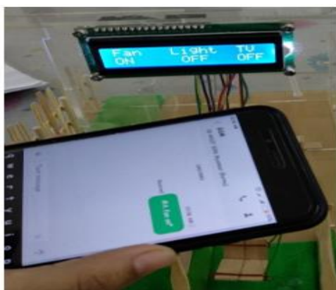
Figure. 16 Photograph of Circuit Operation (Fan ON, Light OFF and TV OFF)
