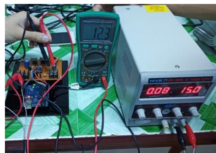
Figure 11. Test and Result of Output Voltage when the Input Voltage is 15V
