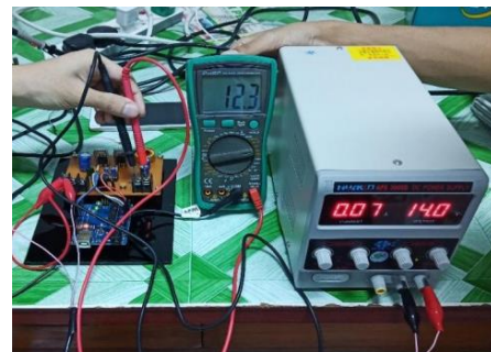
Figure 10. Test and Result of Output Voltage when the Input Voltage is 14V
