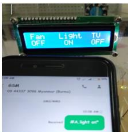
Figure. 15 Photograph of Circuit Operation (Fan OFF, Light ON and TV OFF)
