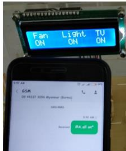
Figure. 12 Photograph of Circuit Operation (All ON)
