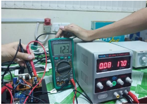
Figure 13. Output Voltage of 12.3V is obtained when 17V Input is supplied
