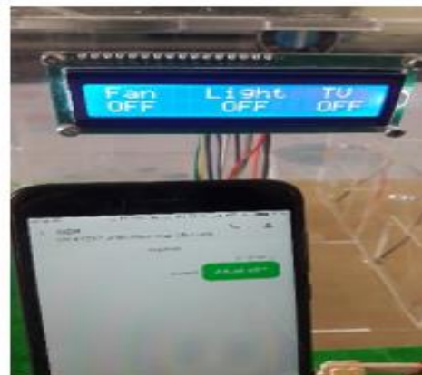
Figure. 13 Photograph of Circuit Operation (All OFF)
