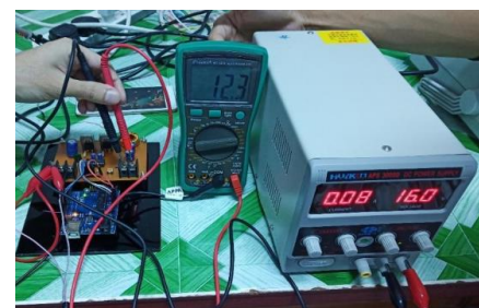
Figure 11. Test and Result of Output Voltage when the Input Voltage is 15V
