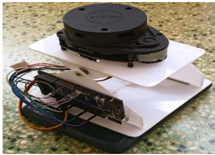
Figure 3. 2D LiDAR configuration with the instruments
