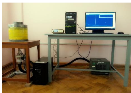
Figure 4. Experimental Arrangement for HPGe Detection System
