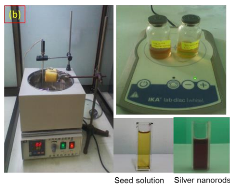
Figure 1 (a-b). The flow charts and preparation steps of the Ag NRs
