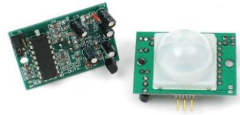
Figure 3. The front side view and back side view of PIR sensor
