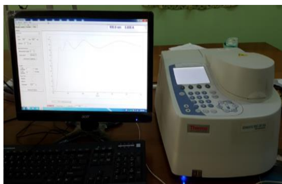
Figure 2. UV-Vis Spectrophotometer (GENESYS 10S)
