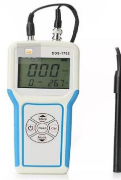
Figure 4. Portable Digital Conductivity Meter
