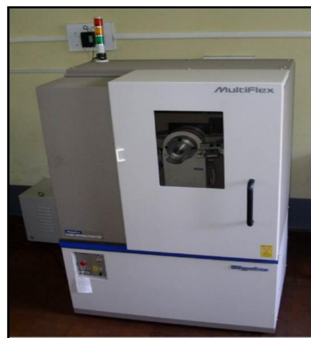
Figure 4 The photograph of the RIGAKU-RINT 2000 X-ray Diffractometer
