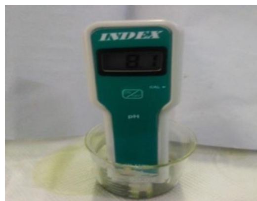
Figure 7. Measurement of pH on Rhinacanthus nasutus Leaves Dye Solution
