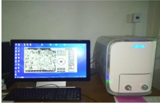
Figure 5. Photograph of JEOL-6000 Scanning Electron Microscope
