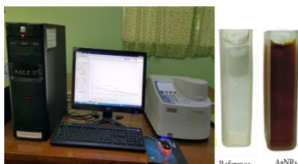
Figure 3. UV-Vis Spectrophotometry (GENESYS 10S)
